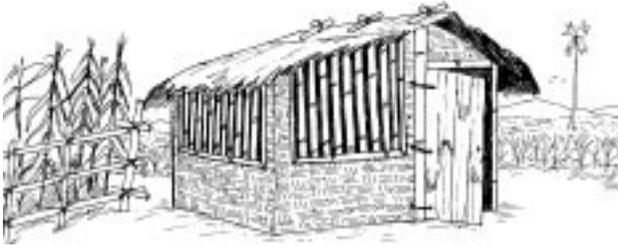
← Solid construction of walls. Made of bamboo, timber, off-cuts, old metal-sheets or sticks with clay.
