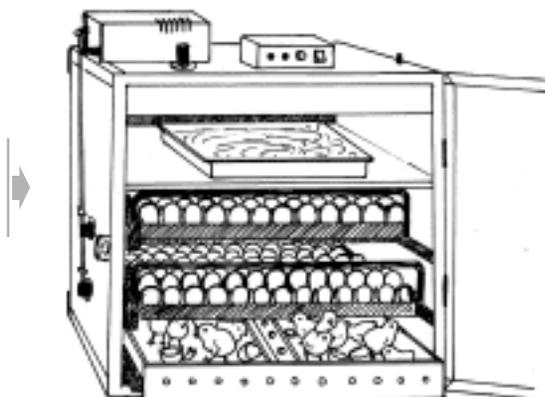
*The setting-trays keep the fertilized eggs from 0 till 18 days. The trays need to be turned regularly (at least once every 4 hours), manually or automatically. The temperature should be kept constant between 37.5 to 38.5 °C with a humidity of around 55%. It is advisable to put new eggs in batches in the incubator, like every 5 or 7 days.*
