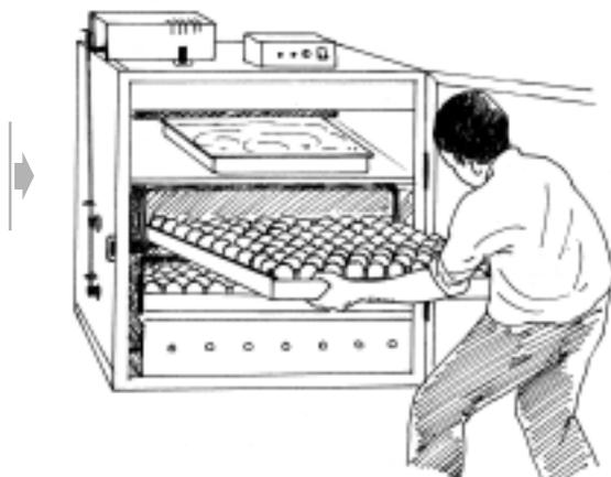
*Close to hatching, the eggs are moved from the setters to the hatching tray to stay from 18 till 21 days (till hatching). In big incubators with a separate hatching compartment, the humidity is increased to around 80%.*
