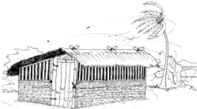
Protection against rain is achieved by a well constructed roof with overhang, made of thick thatch or galvanized iron-sheets.
