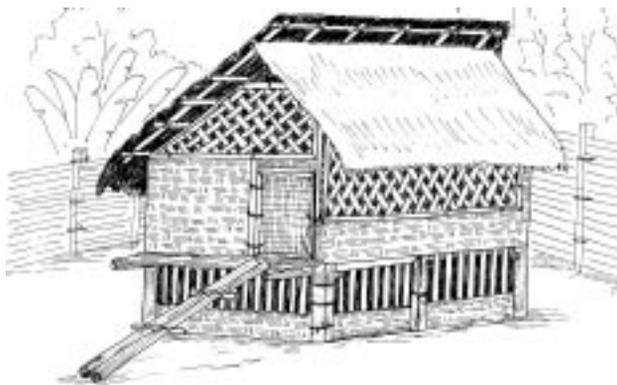
This type of housing is an alternative to the earth floor with litter. The house is on stilts with slatted floor of wood or bamboo (1 cm thick bamboo sticks, with 1-2 cm space in between). The space under the house, where the manure falls, must be fenced so that the chicken cannot go there.
